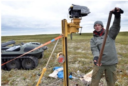
Using an engine to core the tundra peat.
